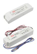
**LED-DR30-12 6-30W** (non-dimming), 1-27W (PWM dimming) 12V DC constant voltage hardwire driver, Class 2, RoHS compliant 100-240AC 50/60Hz input via built-in terminal block with strain relief screw-down cover If used with AL-PWM-6A (see page 208), the dimmer will consume ±3W internally c/UR/us Recognized for indoor use only 6-1/4"L x 1-3/4"W x 1-3/16"H
