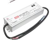
**LED-DR150-24 30-150W** (non-dimming) 1-147W (PWM dimming) 24V DC constant voltage hardwire driver, RoHS compliant 100-240AC 50/60Hz input via 10" 18AWG SJTW conductors If used with AL-PWM-6A (see page 208), the dimmer will consume ±3W internally and will require a repeater for loads greater than 6A (72W at 12V) c/UR/us Recognized for wet or dry locations, 9"L x 2-5/8"W x 1-1/2"H
